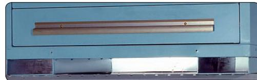
An integral fork lift base consisting of two 1 3/4" x 6" lifting channels arc-welded to the frame itself, permits inserting truck forks into wide channels for safe, easy transport of cabinets - even when fully loaded!
